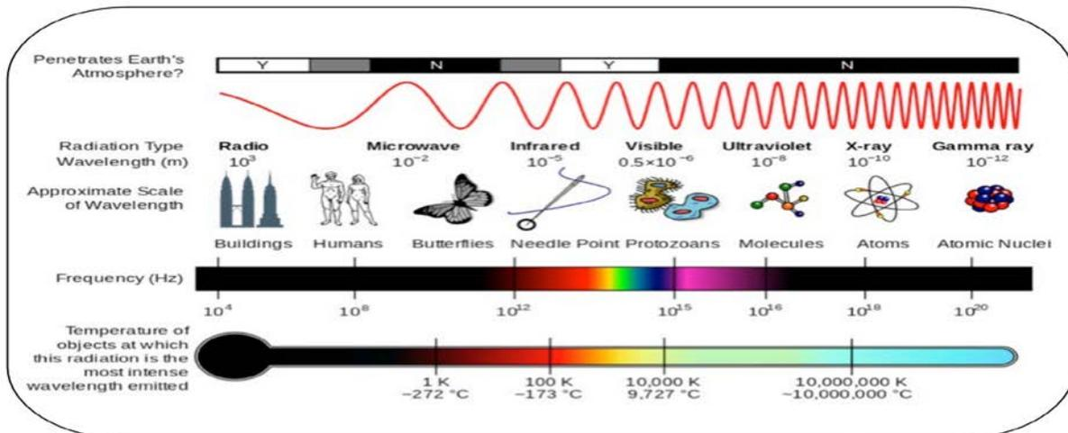
Figure 7: The properties of the electromagnetic spectrum. Credit: Wikimedia Commons.
