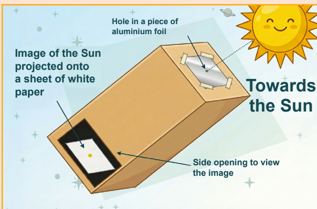
General diagram of a pinhole camera with a side viewfinder
