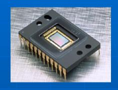
CCDs are detectors made our of silicon. Each element is a pixel (picture element).
