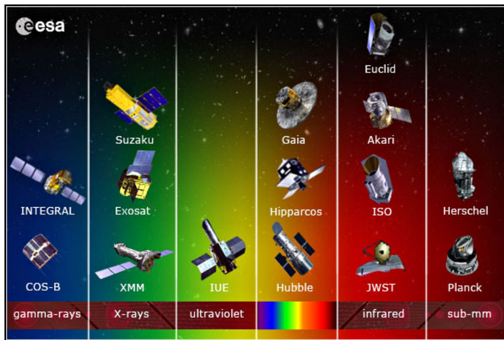
Figure 4: ESA's fleet of telescopes across the electromagnetic spectrum. (The sub-millimetre range corresponds to the shortest radio waves.) Credit: ESA
