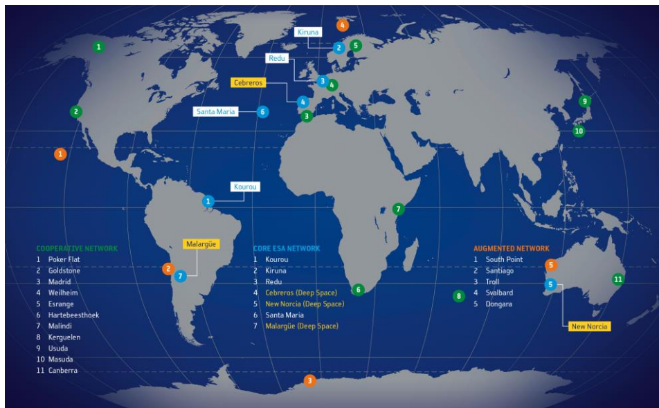
Figure 2 : Tracking antennas used by ESA. (Credits: ESA)
