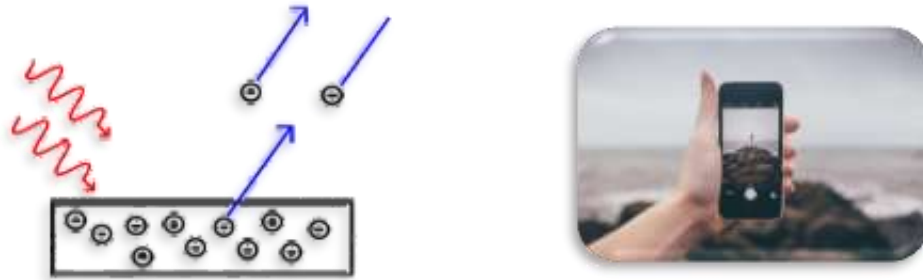
Figure 18: (left) Simplified version of the photoelectric effect, (right) Cell phone camera. (Credit: Wikipedia)
